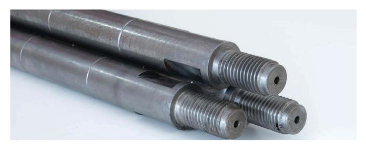
The dynamic probing technique involves driving a rod, marked at 100mm intervals, with a cone attached to the base vertically into the ground. The number of blows for each 100mm of penetration are recorded to measure soil resistance and quality.
