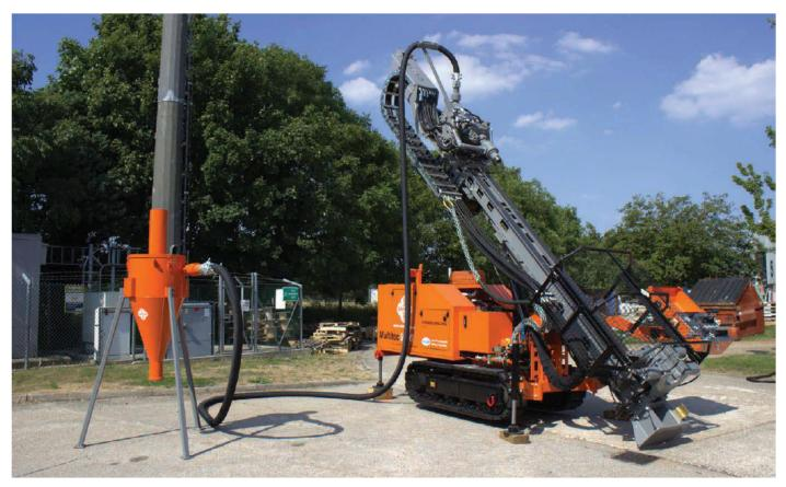
Unlike conventional down-the-hole (DTH) hammers which send the air flush through the centre of the drill string and the cuttings being forced up the hole outside of the hammer and drill rods, reverse circulation does exactly the opposite.
