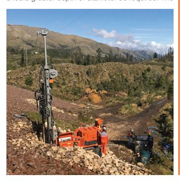
Corani drillers run 3m long drill rods and a swing out mast extension lets them trip two rods at a time in lengths of 6m to save time.
