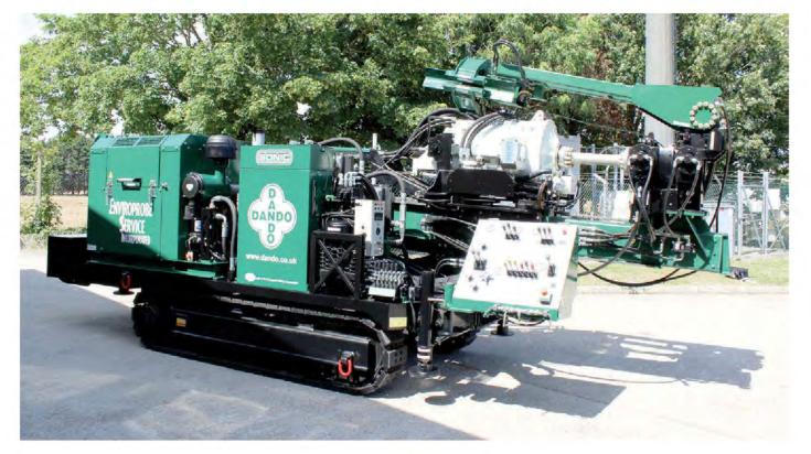
The entire SDC375 drill rig can fit inside a 40foot ocean container, which is ideal considering demand for the machine is expected to expand globally.
