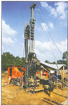
Above: the Multitec 9000, a mid-size rig capable of drilling HQ to over 800m
