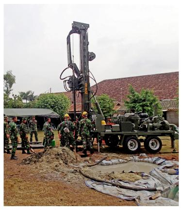
Capable of performing various drilling techniques including mud rotary, DTH and flooded reverse circulation.
