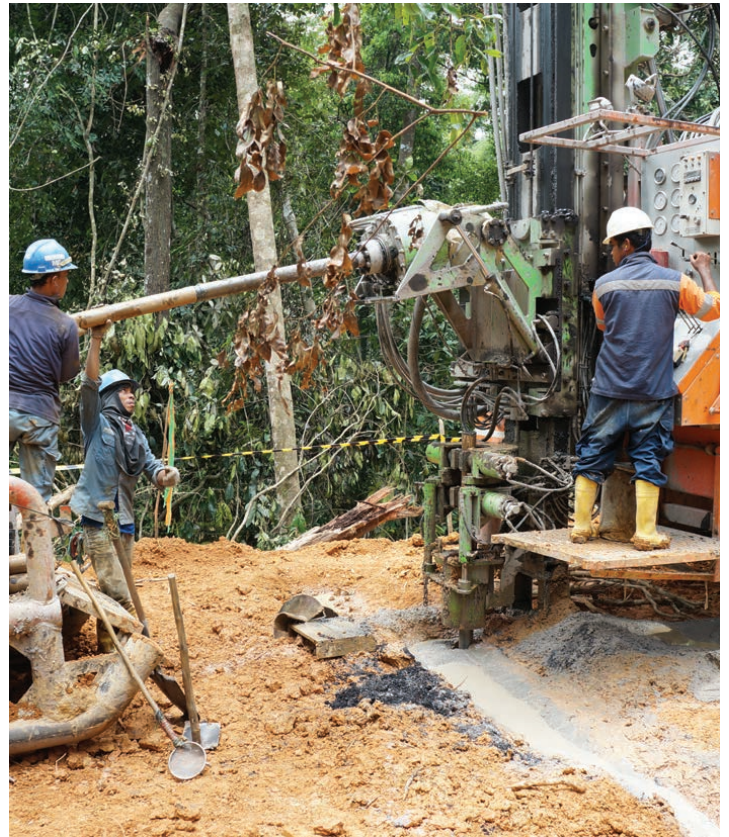
Head tilt for loading roads, and hydraulic side shift for tripping out of the hole.
