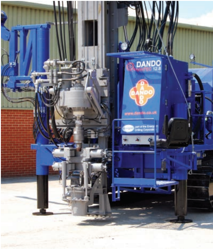
Location of drilling controls provides the driller optimum view of the borehole. High specification rotary heads and double clamps available.
