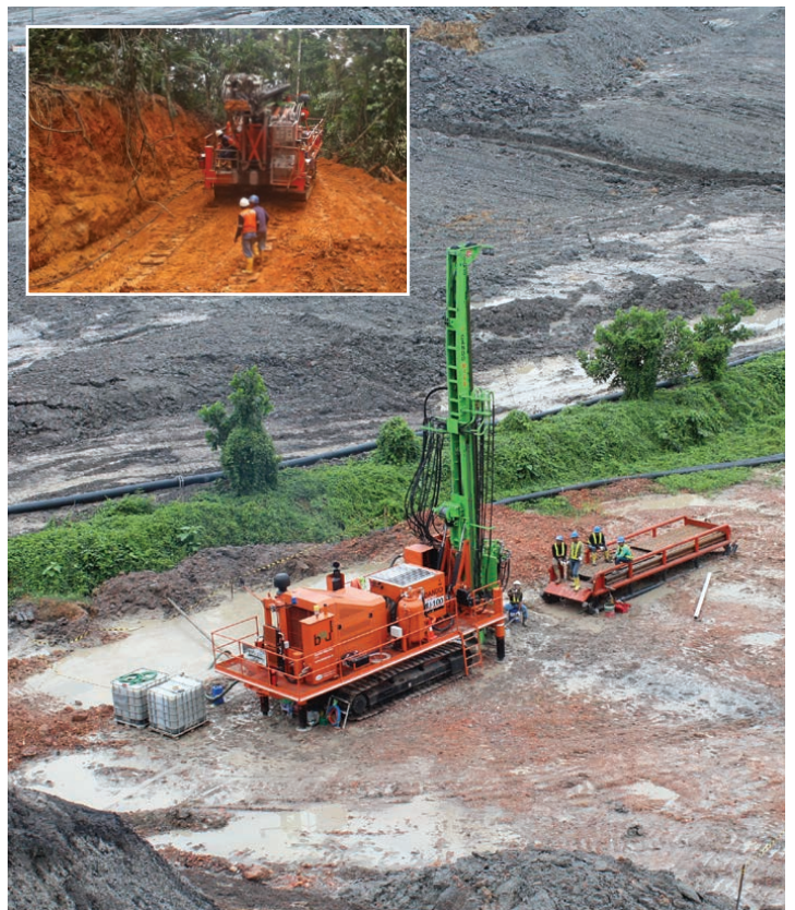
Various mounting options including steel single grouser tracks for when encountering rough, muddy terrain or 6 x 6 truck for quick mobilisation between sites of long distance.
