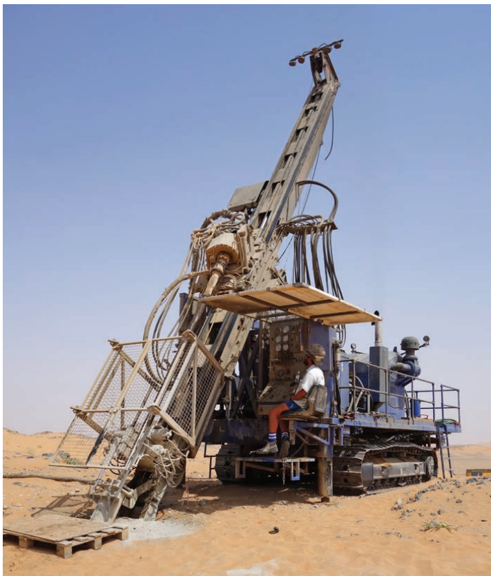
Features include mast dump for angle drilling; main winch for tool handling; wireline winch; double clamps and on-board coring pump.
