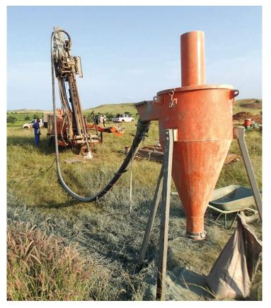
Capable of performing various drilling techniques including RC, RAB, conventional mud, auger, diamond wireline coring, SPT, geothermal heat pump drilling and more.
