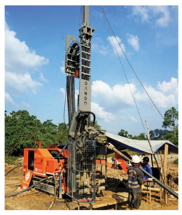
4 speed rotary head mounted to a hydraulic side shift with optional floating spindle. Hydraulic head tilt available. Various head options.
