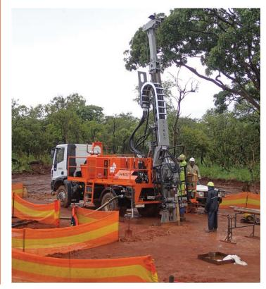
Various mounting options available including tracks for when encountering rough, muddy terrain or 4 x 4 truck for quick mobilisation between sites of long distance. Trailer mounted is also an option.
