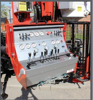
Uncomplicated and user friendly swing out control panel with ergonomic layout and LED console lighting.
