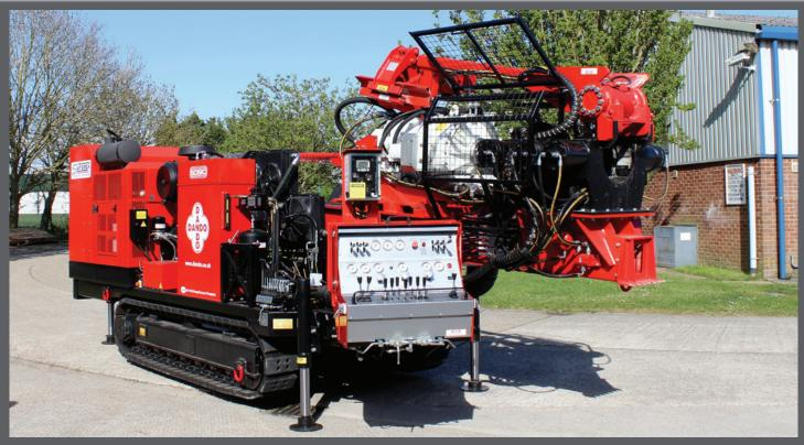
Compact crawler mounted design ideal for maneuvering through tight areas of difficult access. The rig is available with multiple track options as well as truck mounting.
