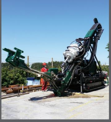
Mast dump allows drilling to be conducted at angles of up to 45 degrees.
