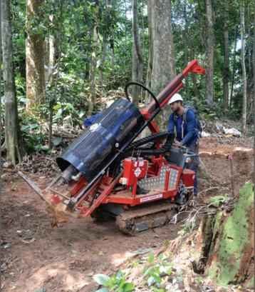
The Terrier's ultra-small footprint and easy maneuvrability means the rig causes very little disturbance to its surroundings.
