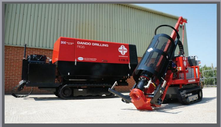
The Angle Drilling Terrier is available supplied with a track mounted compressor providing 400 cfm at 145 psi.
