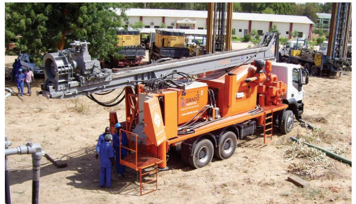
High torque rotary head with hydraulic side shift and head tilt.
