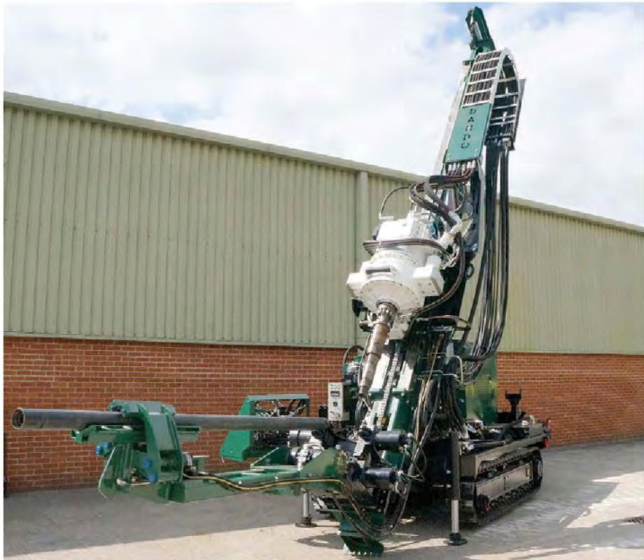
Enviroprobe's Dando SDC375 is fitted with a single-rod loader, which uses the most powerful Sonicor 50K head. Source: Dando Drilling photos
