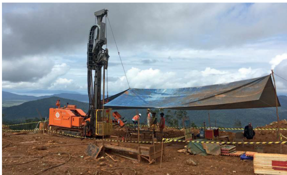
Dando's top drive rotary Jackal rig being used for nickel exploration in a remote part of Sulawesi
