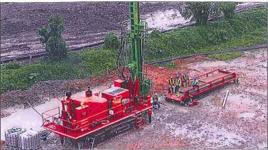
for copper exploration, the Multitec 9000 was conducting wire-line core drilling using HQ rods in the Zambian bush. Mounted on tracks and with a small footprint, the Multitec 9000 is meant for drilling in remote areas of difficult access.
