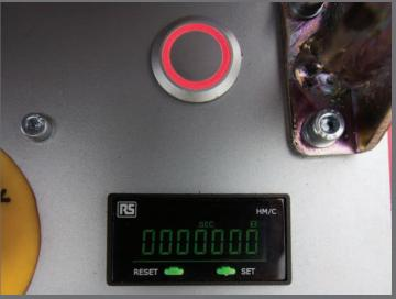
Hydraulic stabilising legs allow faster deployment SPT blow counter with illuminated digital display and large reset button.
