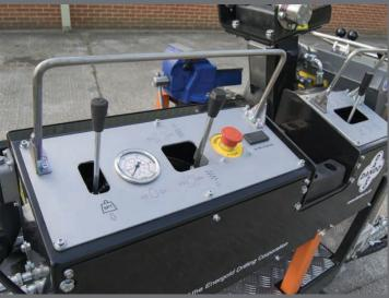
Revised control console complete with emergency stop and pressure gauge positioned towards front of the rig for good visibility of the borehole.
