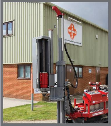
Trip hammer swings out from the drill line at any Cantripout multiple rods for increased productivity. of casing without moving the rig.
