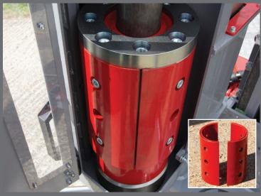
New split weight design. 63.5kg reduced to 50kg with the removal of only 8 bolts. No additional brackets to reduce drop height from 760-500mm.
