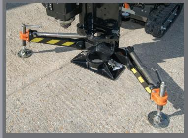
Lightweight, folding stabiliser legs with ball jointed adjustable jack feet. Hydraulic option also available.
