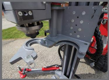
Swing-out pullback ring allows open access to the borehole.
