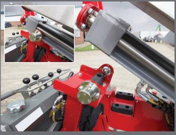
Mast automatically locks into headache post with no additional pins for road transportation.
